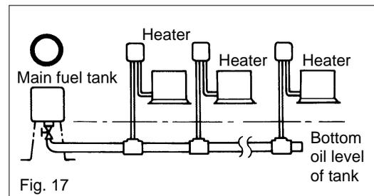
(b) The large diameter horizontal piping should not be installed at a higher level than the bottom of the fuel tank. As it will cause the pumps to overload and require excessive time for suction or the lifter to be incapable of suction. (Fig. 18)
