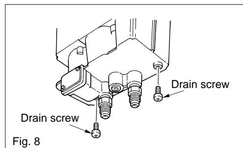
Note: To catch the fuel and water that will drain out, set a half gallon container under the unit.
