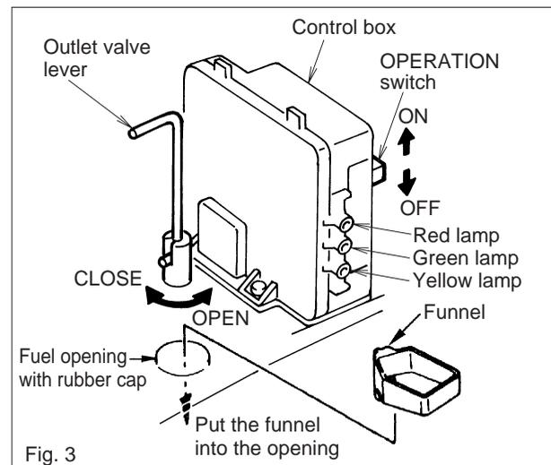
4. Turn the operation switch to ON position. The green lamp will change from flashing to continuous and the motor will start operating.
