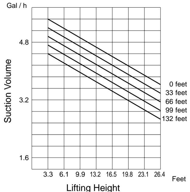
Note: The lifting pipe is a 3/8" OD copper pipe.
