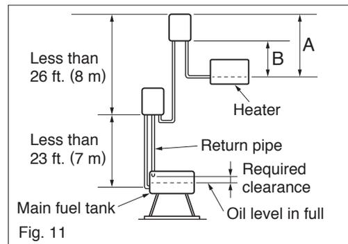
(b) Be sure to install a return pipe for operating with series-connected lifters. Install the return pipe in such a manner that there will be a clearance provided between the outlet of the return pipe and the full oil level line in the main fuel tank. (Fig. 11)
