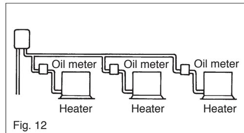
CAUTION: Sufficient care should also be taken when installing more than four oil meters, which may jeopardize the lifter to overfill and leak oil.
