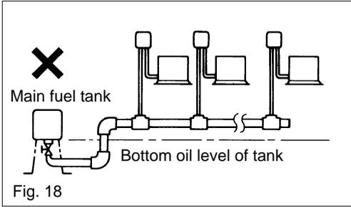
2. The amount fuel remaining inside the outlet line must be less than 1.3 gallons (5 liters).
