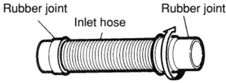
11. Pass the hose band for standard flue pipe set, which is attached to the unit, through one of the rubber joints, next connect the rubber joint into the air intake mouth of the flue pipe, and then secure the piping with the hose band.
