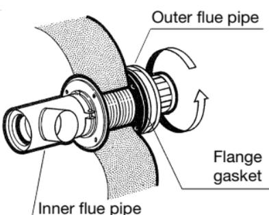
7. Insert the flexible exhaust pipe to the flexible bent joint until it locks. Insert the flexible bent joint to the exhaust mouth of the inner flue pipe until it locks.
