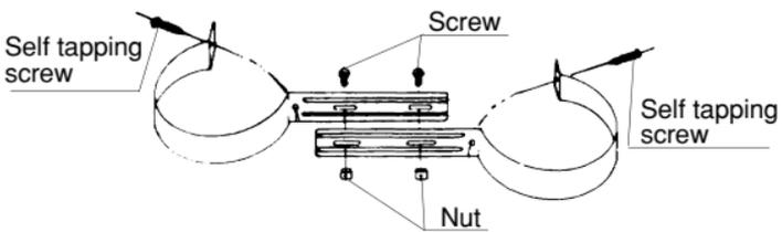
If the clearance between the extension pipe "A" and "B", is too wide, cut the pipe support bracket to the appropriate size.
