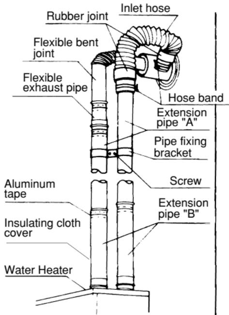
15. After assembling the parts as above, do a trial operation to the Water Heater and check to see if it works properly and that there are not any emission leaks from the joints.
