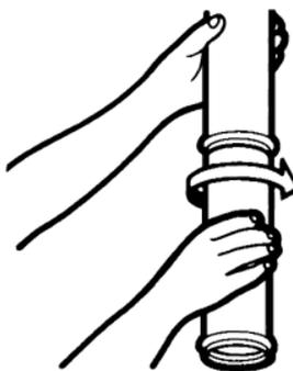
9. Remove the screw from the exhaust mouth of the unit. Insert the flexible exhaust pipe to the exhaust mouth and secure them with the screw.
