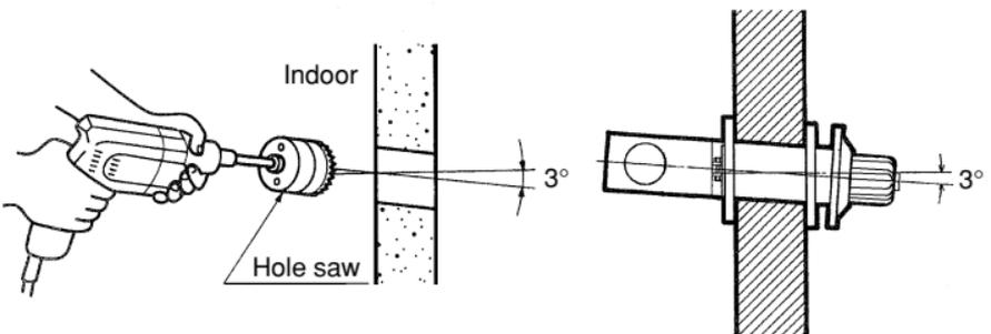
5. Install the inner flange and the flange gasket to the inner flue pipe and insert the inner flue pipe through the wall hole from inside the room. Make sure the arrow on the inner flange is pointing up and secure the securing band with a screw and a nut through two holes of the locking band. Secure the inner flue pipe to the wall with the four screws provided with the unit.
