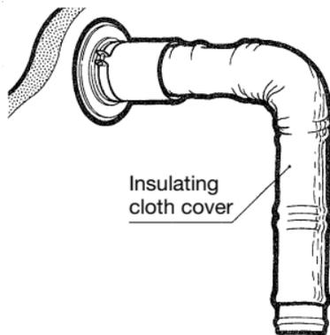
2. When disconnecting the extension pipe (such as flexible pipe and flexible elbow), pull the pipe by turning the pipe clockwise.
