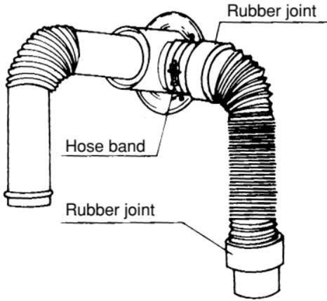
12. Next pass the hose band through the other rubber joint and then secure the extension pipe "A", which has been connected to the air intake mouth of the Water Heater, with the hose band.
