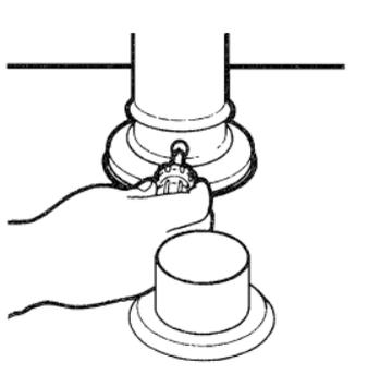
10. Connect rubber joints to both ends of the inlet hose.
